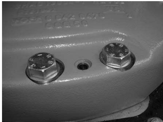
Figure 11 Four \varnothing 12 H8 (depth 12) on radius 400 mm from axis 1 center on robot base.
