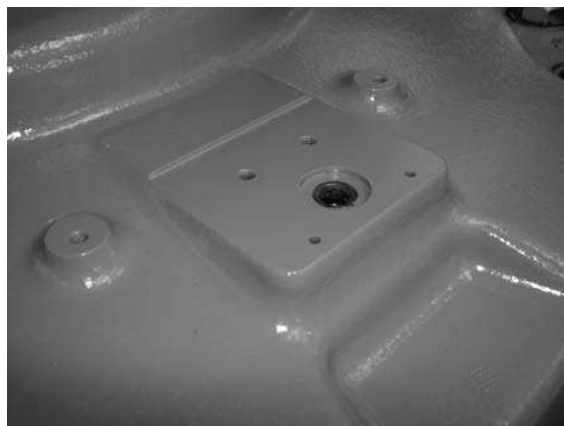
Figure 11 Four \varnothing 12 H8 (depth 12) on radius 400 mm from axis 1 center on robot base.
