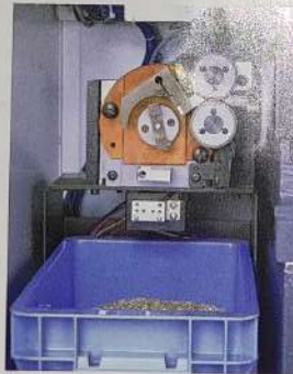
Used wire collector
