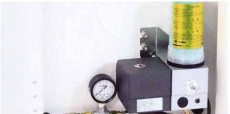
Automatic grease lubrication
