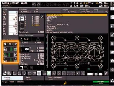
Touching the buttons to adjust the EDM parameters
