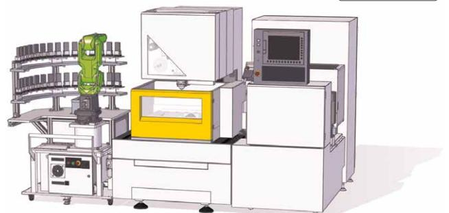
Work piece exchange system by FANUC Robot (sample)
