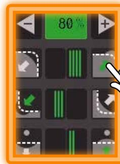
The cutting speed can be adjusted from 50% to 120% keeping the discharge gap to achieve stable cutting
