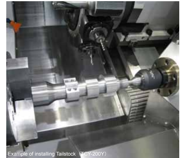
Example of installing Tailstock (TCY-200Y)
