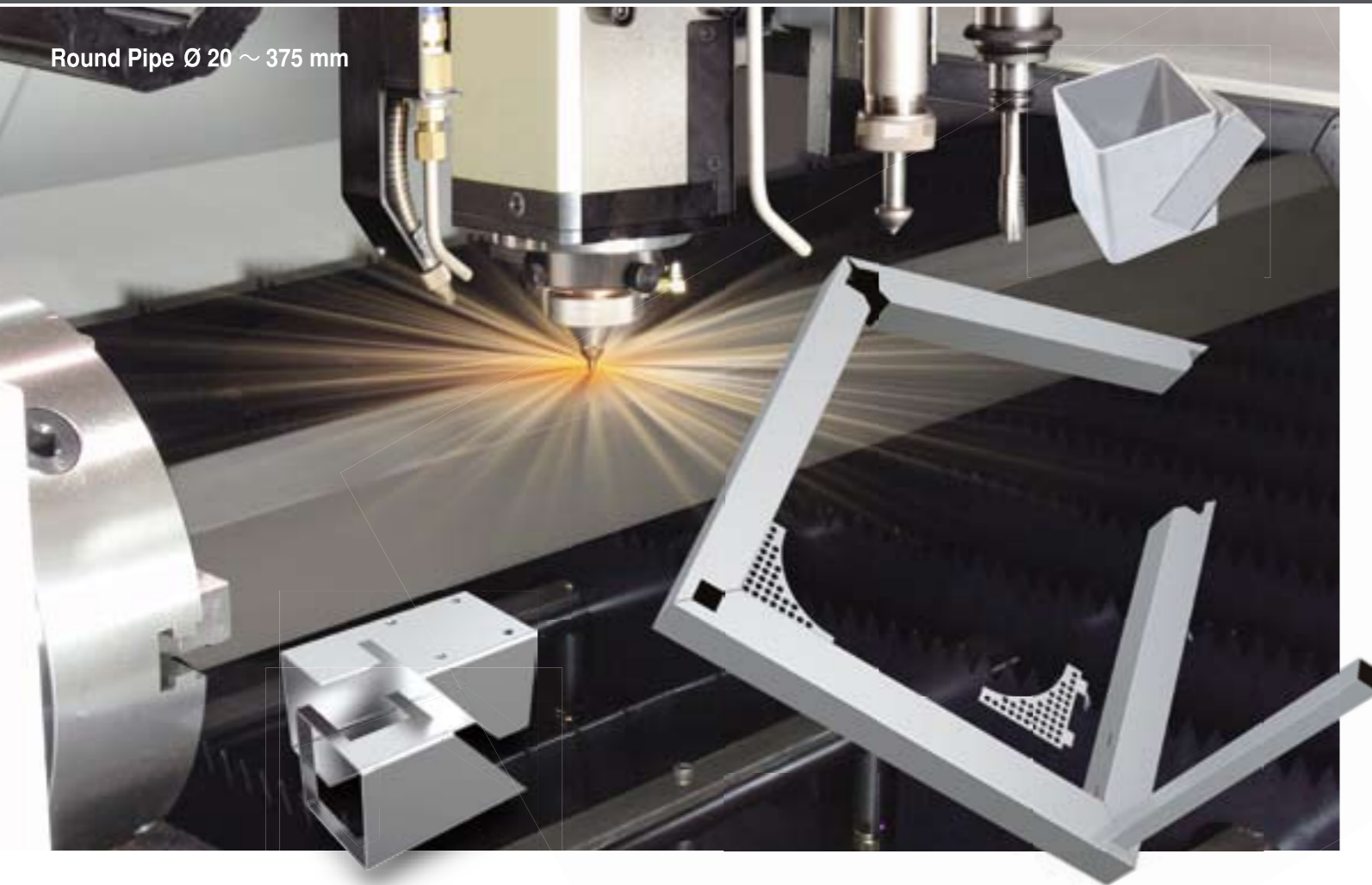
When changing cutting from flat worksheets to pipe processing, the cutting torch is changed
