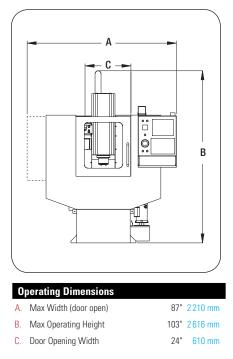
Machine depth is 85" (2159 mm) and requires additional 36" (914 mm) to open rear service panel.
