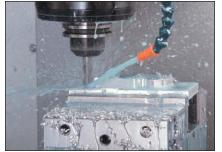
The Mini Mill and Super Mini Mill are perfect for machining the typical small parts found at many job shops. The 40-taper spindle is ideal for finish work and cutting aluminum.
