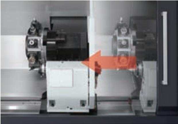
By connecting the tailstock and turret by a pin, the Z-axis can drive the tailstock without using a servo motor.
