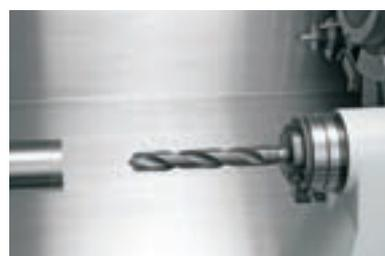
Machining using the tailstock drill (option)
