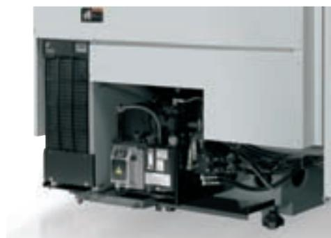
The oil cooler and hydraulic unit are placed together at the rear of the machine without a cover for easy access.
