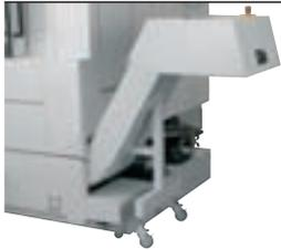
A chip conveyor that efficiently disposes of chips. Choose the specifications right for you.
