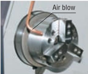
Air blow system, chuck (spindle 1)
