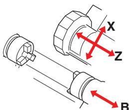
**SMC** Sub-spindle+Milling+C-axis control
