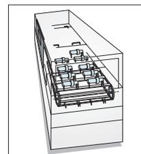
Workstocker for shaft workpieces
