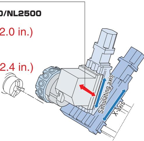
The Y-axis is created by linking the feed of the X-axis and the simulating axes. We have made the axis unit compact and restricted the height of the machine.
