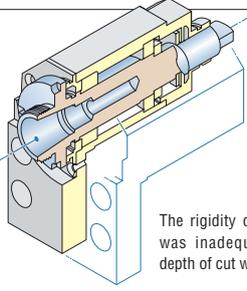
The rigidity of the structure was inadequate when the depth of cut was large.
