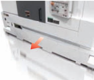
With the new design, the coolant tank can be pulled out in front without having to pull out the chip conveyor. It can be pulled out easily and does not take up extra space in the back.
