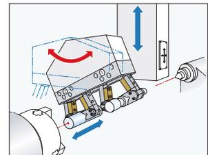
Hand for shaft workpieces
