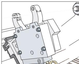
**Hydraulic steady rest (bolt-tightening)** **OP**
