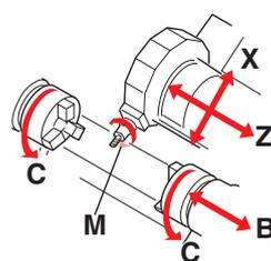
**SY** Sub-spindle+Y-axis control
