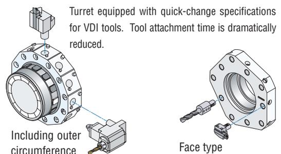
● The face type is only available for 2-axis turning specifications.
