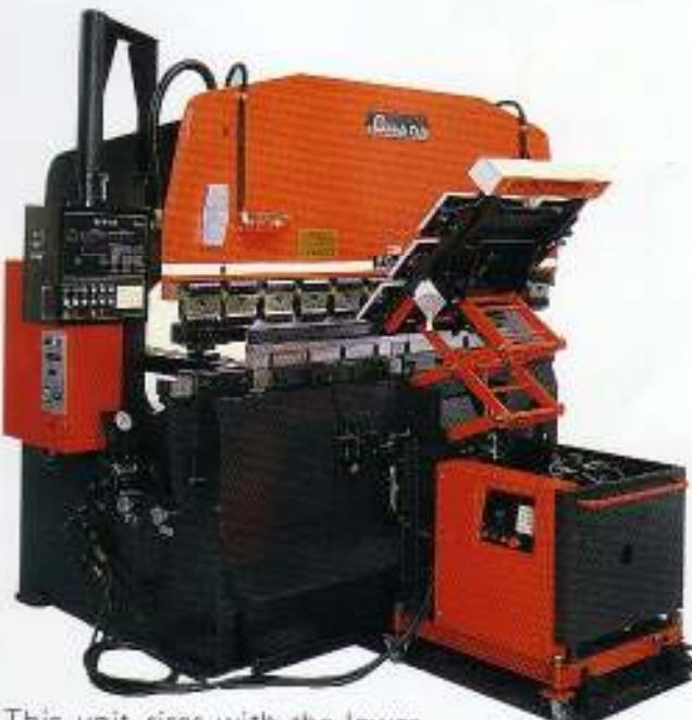
This unit rises with the lower beam of the press brake and supports the workpiece during the bend to prevent distortion.
