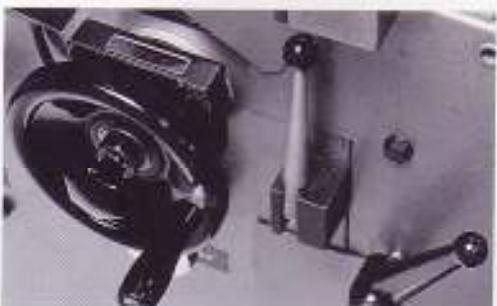
Amada hydraulic press brakes feature the fast approach/slow bend. This protects the operator from sudden workpiece movement and increases production speed. The operator can set the point where the lower beam movement changes from fast to slow with the speed change position setting lever.
