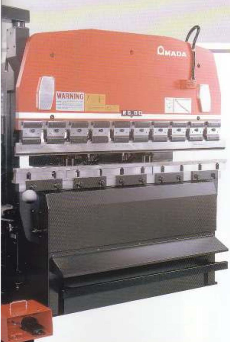
**Roller Bearing Guide Block System Ensures Parallelism for Unprecedented Accuracy.**
