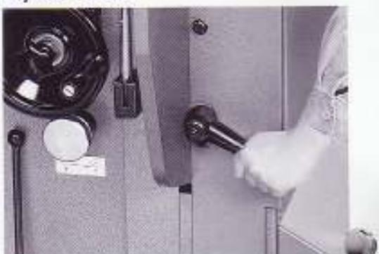
Unnecessarily long bending strokes waste production time and are dangerous and tiring for the operator. The most efficient stroke length can be set by the lower limit setting lever.
