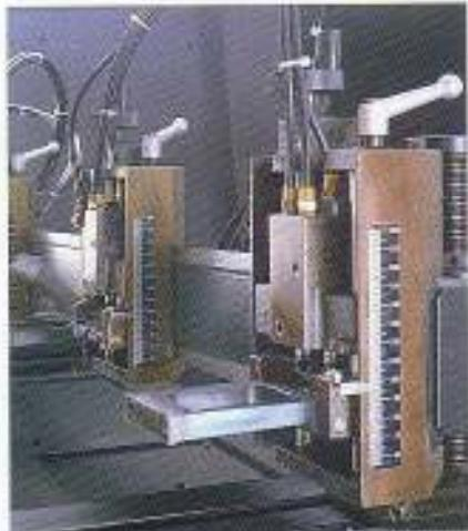
The best for bending longer or shorter sides of the workpiece to complete a box type product. The L-axis is activated with the left and right independent drive systems, so you can position the workpiece at an angle.
