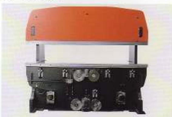
The lower beam moves on pre-loaded bearing guide blocks rather than on conventional friction guides. This entirely eliminates side play or uneven movement by firmly holding the beam parallel at all times. The Amada bearing guide block system is permanently self-lubricated and requires no maintenance at all.
