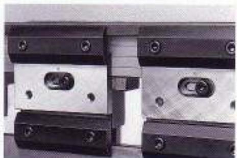
The individual punch holders can be moved as needed to provide access for deep box forming. Window and horn applications can be performed in the center of the machine. Each punch holder has a calibrated wedge for making fine bending angle adjustments.
