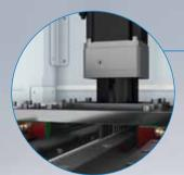
**Impressive precision with rack-and-pinion drive** Rack-and-pinion drive for high-precision robot positioning with fast movements in all axes.
