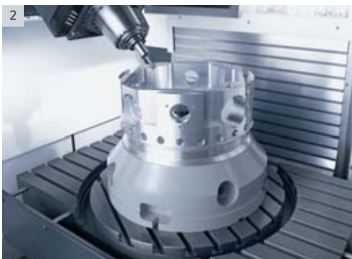
|1| Milling head as an NC controlled B-axis with a swivel range of 150° |2| NC rotary table integrated into the fixed table |3| NC indexing head with cylindrical head machining |4| Vane manufacturing on the BLADE table |5| Cylinder head machining
