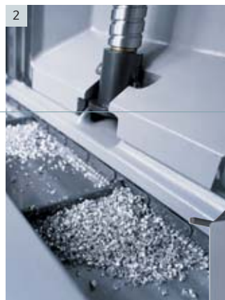
1|1 Optimised tool magazine for 24 or 32 tools in the standard version 1|2 Integrated scraper-belt chip conveyor in the standard version
