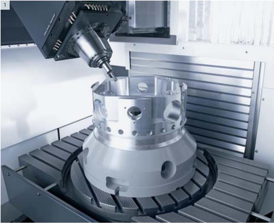
1| Large work area with an integrated NC rotary table and NC controlled milling head (optional) 2| Machining with a B-axis and negative angles
